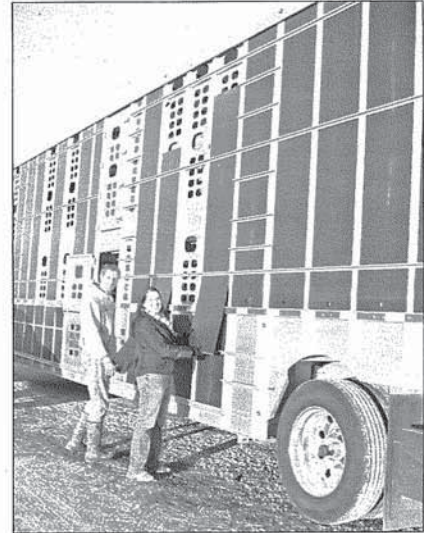
RICK REICH , owner Reich Trucking, and Dr. Angela Green , University of Illinois assistant professor of Agricultural and Biological Engineering, show how wind boards can be removed and adjusted on a trailer.
